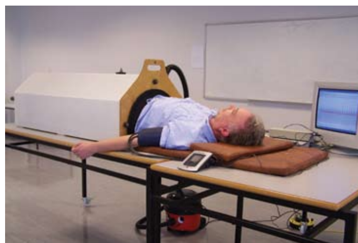
Figure 1: The lower body negative pressure chamber, which is sealed up to the iliac crest of the volunteer.
