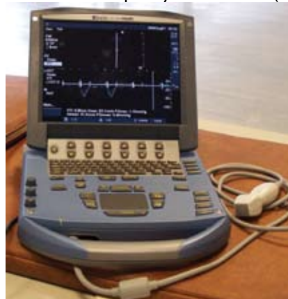
Figure 2: SonoSite MicroMaxx™ portable ultrasound system (SonoSite Ltd, Herts., UK) with the P17 cardiac probe attached. The screen shows a Doppler waveform.
